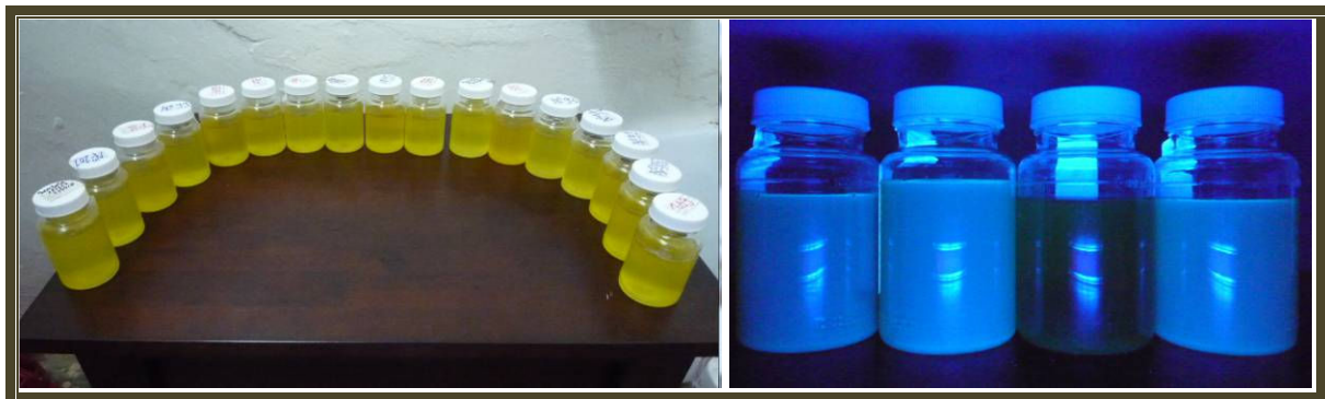
Figure 11: Water testing using colitag test kits
