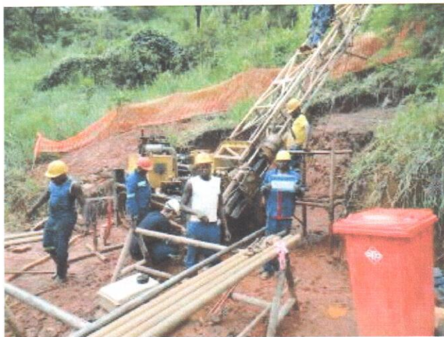
Figure 6 Zani central, Le forage carottant
