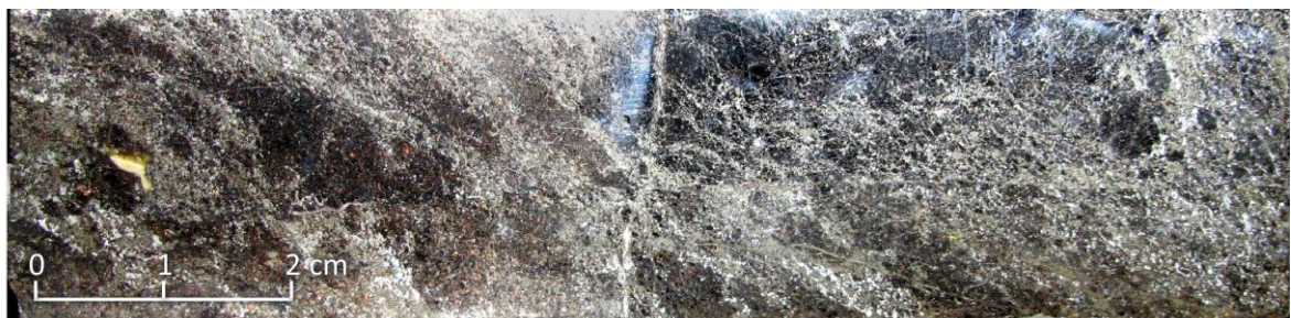
Figure 7-5 Photograph of core showing massive sphalerite (zinc) and galena (lead).
